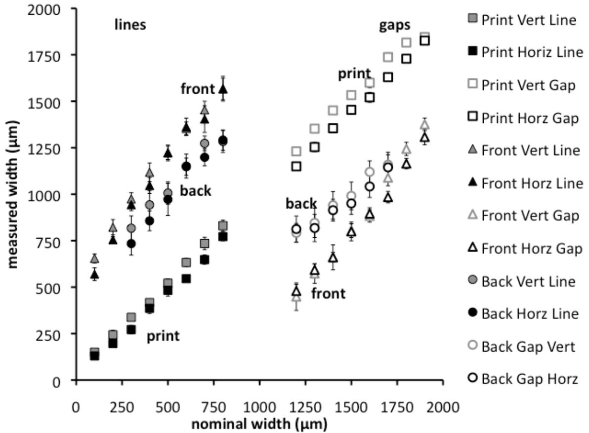
**Figure SI-1.** Measurements of line (barrier) and gaps (channel) widths before (print) and after (front and back) the melting process as a function of the nominal widths defined in the drawing program. The error bars represent one standard deviation ( $n = 10$ ).
