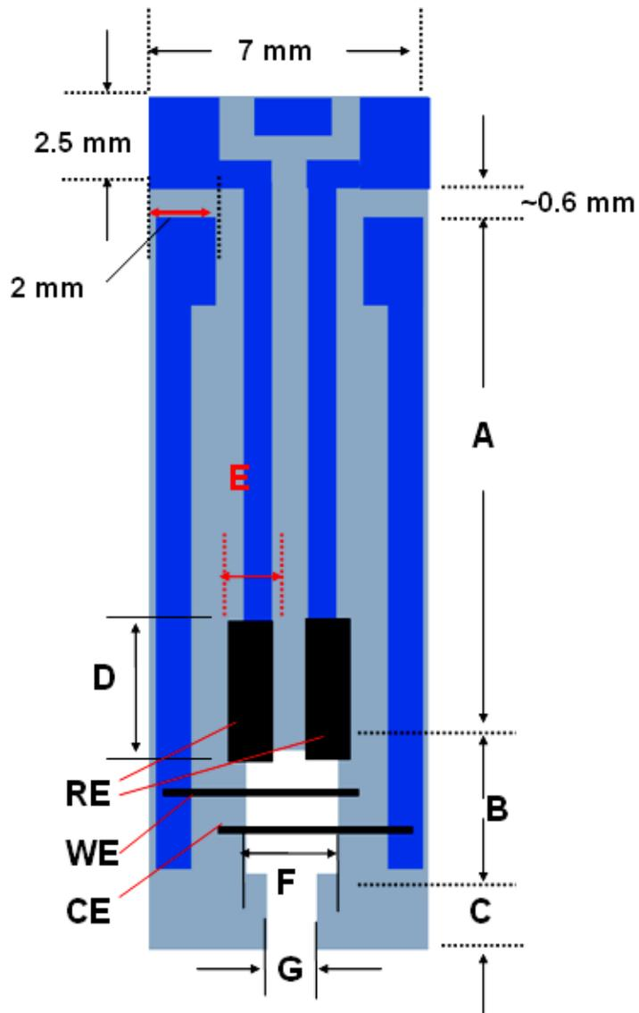
**Table S11.** Dimensions of E $\mu$ PADs Used for the Electrochemical Analysis.
