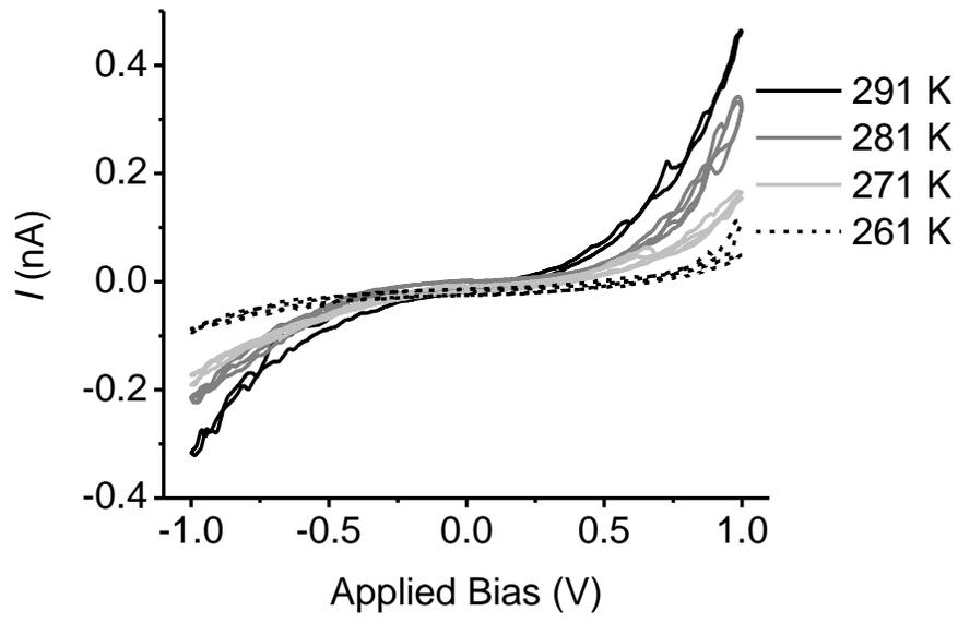
**Figure S4:** An example of  $\text{Ag}^{\text{TS}}\text{-SC}_{11}\text{Fc}_2//\text{Ga}_2\text{O}_3/\text{EGaIn}$  junction that was stable during  $J(V)$  measurement of  $\pm 2.0$  V. This figure shows 9  $J(V)$  traces after which we terminated the experiment.
