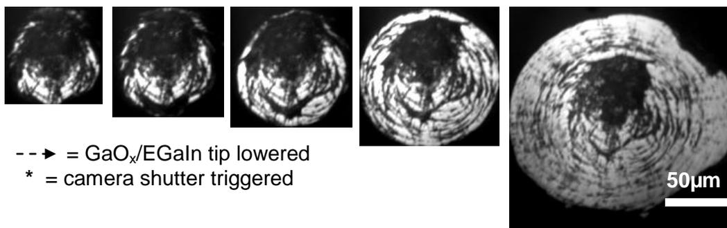
260 K, the liquid EGaIn solidified, disturbing the contact between Cu and Ga<sub>2</sub>O<sub>3</sub> and hindering further measurements.
