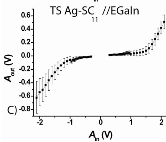
**Figure S2:** An example of  $\text{Ag}^{\text{TS}}\text{-SC}_{11}\text{Fc}_2//\text{Ga}_2\text{O}_3/\text{EGaIn}$  junction that was stable during  $J(V)$  measurement of  $\pm 2.0$  V for nine  $J(V)$  traces after which we terminated the experiment.
