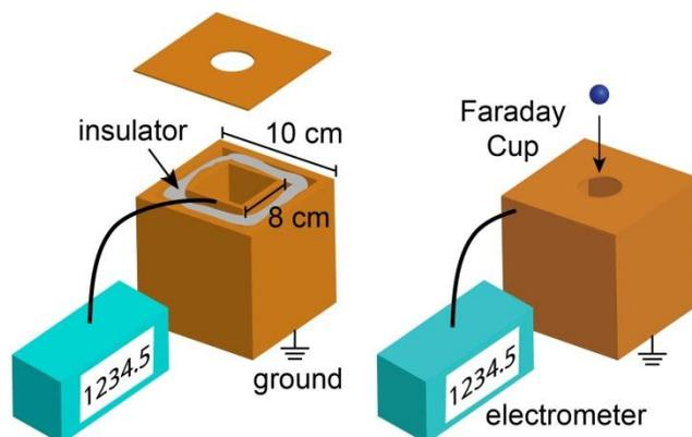
**Figure S1.** Illustration of the Faraday Cup connected to an electrometer
