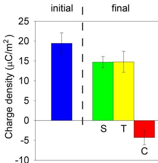
**Figure S4.** Undyed Nylon beads demonstrate similar behavior of contact de-electrification. After contact, the center bead discharged (S = side bead; T = top bead; C = center bead).
