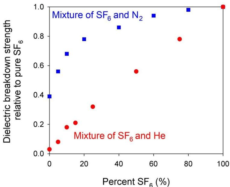
Figure S6. Dielectric breakdown strength of a mixture of sulfur hexafluoride (SF<sub>6</sub>) and nitrogen (N<sub>2</sub>) or helium (He). (Data taken from Table 6.11 of ref <sup>2</sup>)
