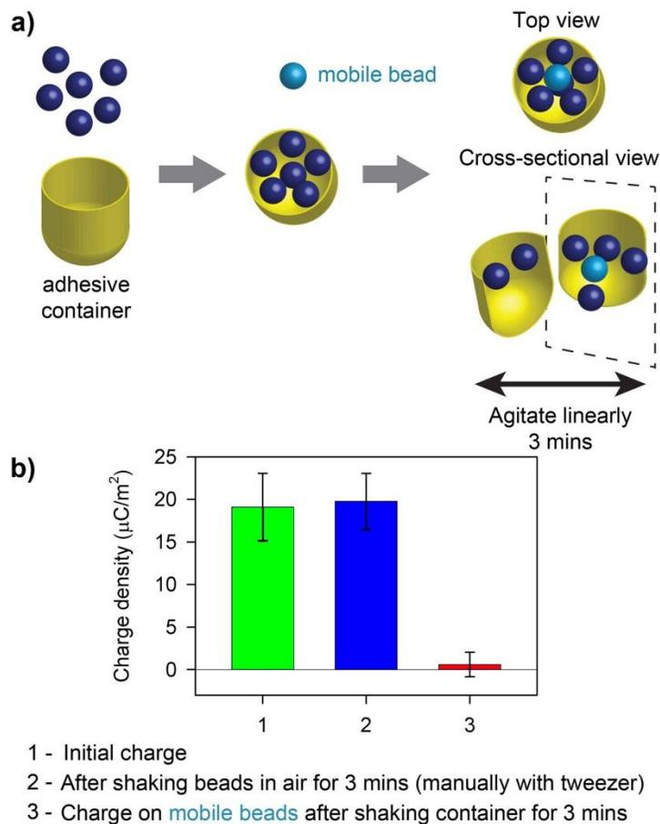
**Figure S5** An alternate experimental setup for observing contact de-electrification. (a) Six already-charged Nylon beads were placed in a container with adhesive interior, so that they were fixed in position. The first bead was placed at the bottom of the container, whereas the five other beads were fixed above the first bead and onto the sides of the container, arranged in a pentagon. A seventh Nylon bead (the “mobile bead”, colored light blue for clarity) was inserted loosely in
