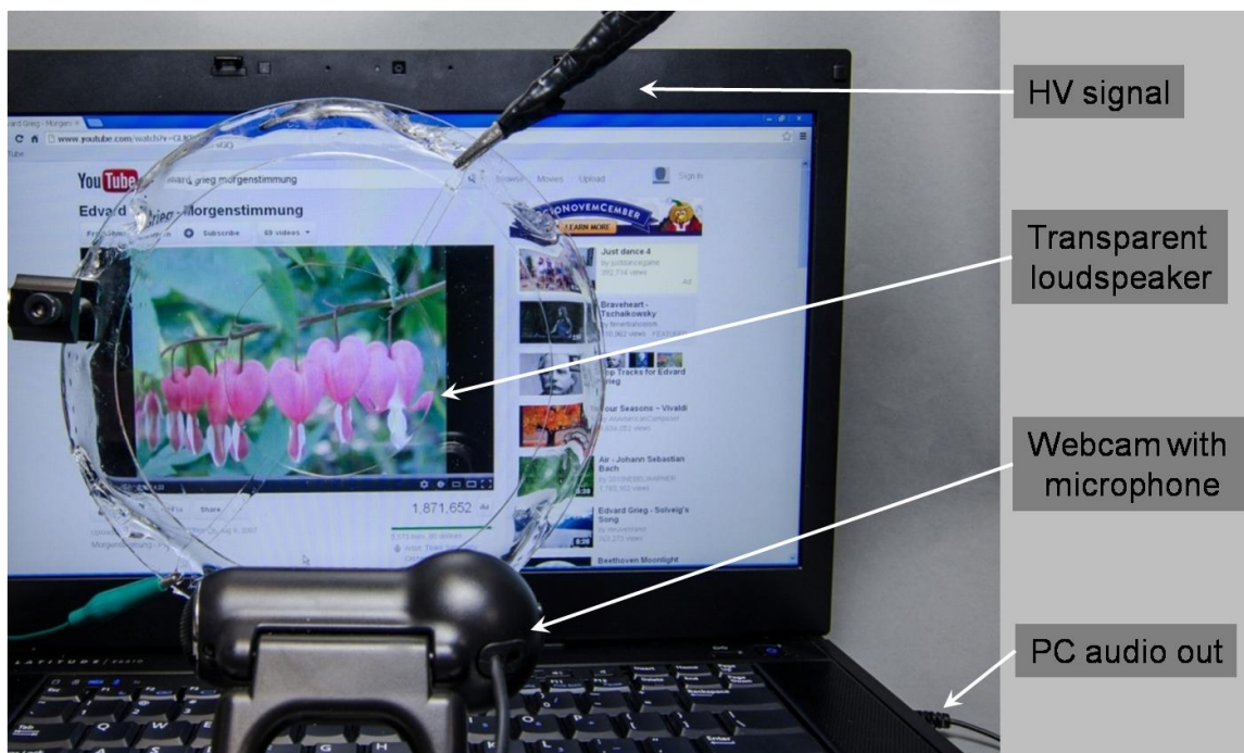
Fig. S5. The experimental setup for the transparent loudspeaker. The loudspeaker is placed in front of a laptop playing a music video. The video is clearly visible through the loudspeaker. The sound track of the video is fed to the loudspeaker as a high-voltage signal, from the audio output of the laptop, through a high voltage amplifier. A microphone records the sound produced by the loudspeaker.
