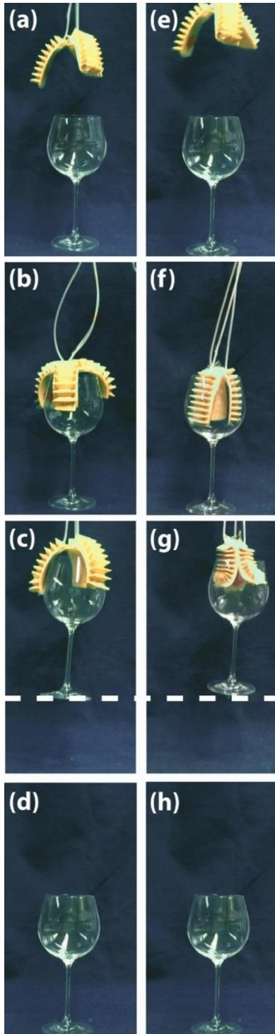
**Figure 3.** (a) A composite material, bellows-like actuator that (b) bends when pressurized. (c) The material seals around a puncture and the actuator continues to function, (d) even when the source of puncture (a 14 gauge needle) is removed. Scalebar is 2 cm.
