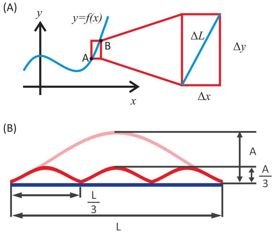
**Figure S4.** (A) The arc length of an arbitrary function,  $f(x)$  from  $A$  to  $B$  can be described as an equation using the Pythagorean Theorem. (B) The amplitude of a longer sheet (red) decreases proportionally to its wavelength (one third in this exemplary diagram) when the total arc length is constant.
