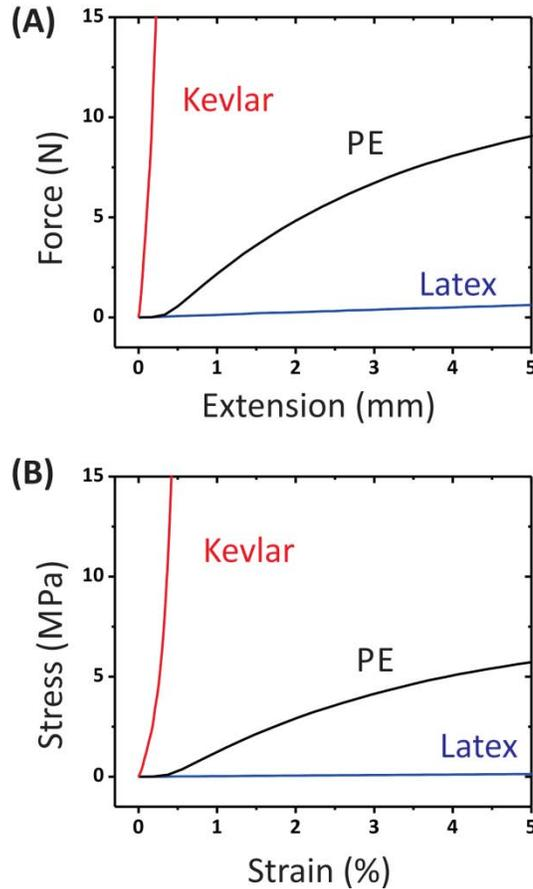
**Figure S1.** Force vs. extension and stress vs. strain curves of Kevlar, PE and latex strips. The size of the strips tested was 30 mm in width and 90 mm in length. The Young's modulus of the three materials differed by four orders of magnitude (2.7 MPa, 55 MPa and 24 GPa).
