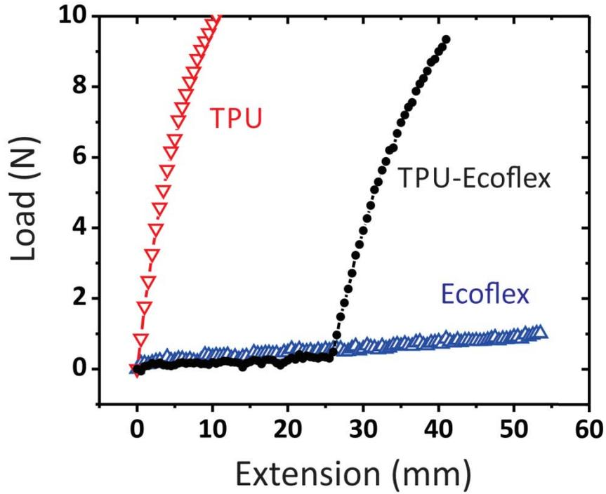
**Figure S2.** Force vs. extension curves of a silicone-based elastomer (Ecoflex), thermoplastic polyurethane (TPU), and a TPU-Ecoflex stepped modulus composite. The length difference of the strips of TPU and Ecoflex of the composite was 25 mm. The measured Young's moduli of Ecoflex and TPU are 44.2 kPa and 17.7 MPa.
