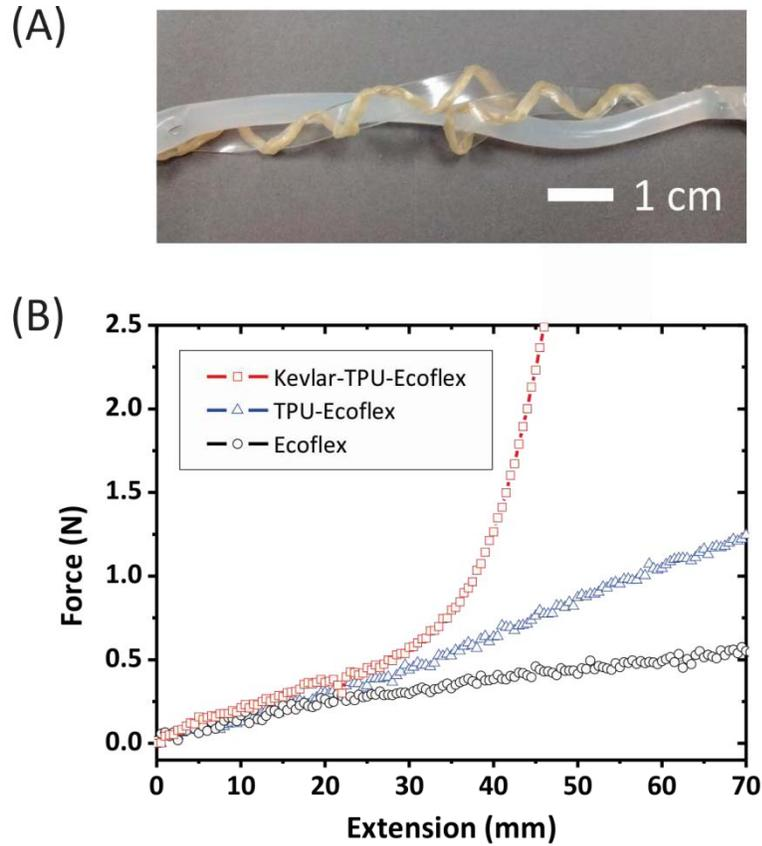
**Figure S7.** (A) Photograph of a Kevlar-TPU-Ecoflex composite with rod-coil configuration. The TPU strip was wrapped with Kevlar fibers in a helical fashion; this TPU-Kevlar composite was wrapped around a rod of Ecoflex. (B) Force-extension profiles of a Kevlar-TPU-Ecoflex (□) and a TPU-Ecoflex (Δ) composites, and a single rod of Ecoflex (○).
