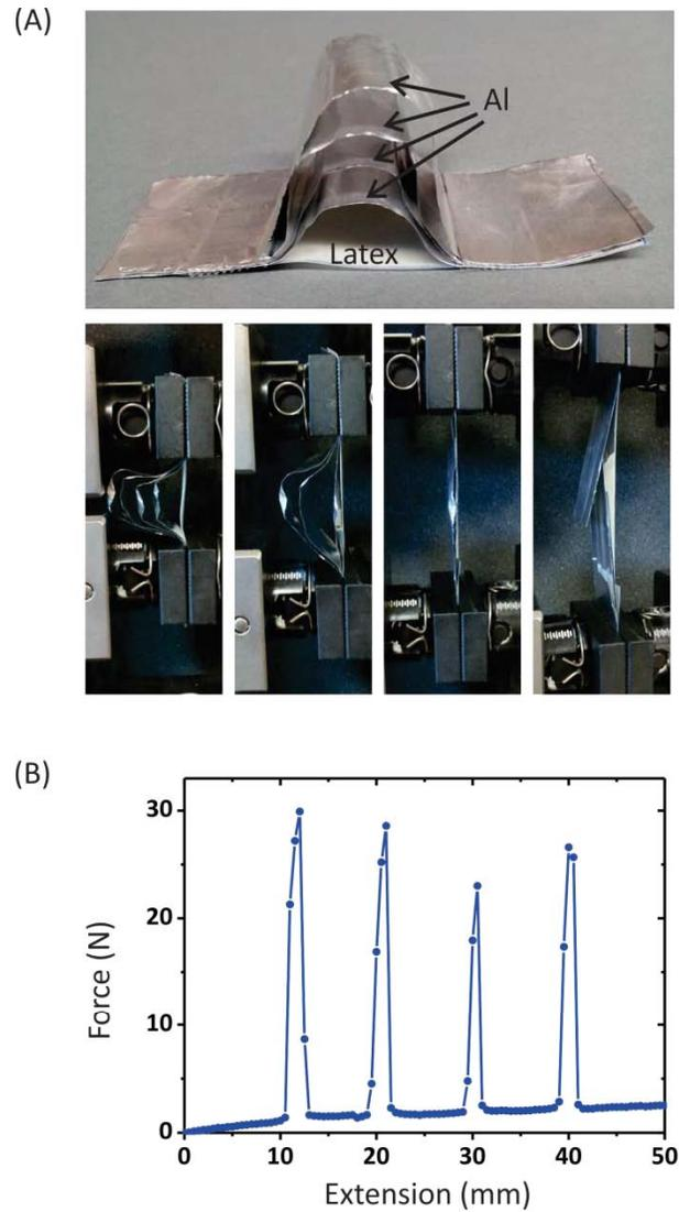
**Figure S3.** (A) Layered composites of four sheets of aluminium and a layer of latex at rest (top) and in tensile strain (bottom). (B) The force-extension of the composite shows sharp peaks at four threshold extensions that are 10, 20, 30 and 40 mm as the Al layers break from the shortest to the longest. The latex layer helps the shortest Al layer maintain its wavy configuration at rest and prevents the composite from totally separated into two pieces even after the longest Al layer breaks.
