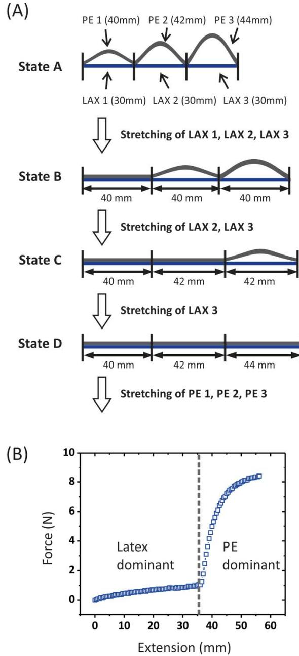
**Figure S5.** (A) Four states of a stepped modulus composite with three sections of different arc length when the applied strain increases. Until the state D is reached, only the latex sheet stretches. (B) Force vs. extension curve of a latex-PE stepped modulus composite described in (A). The threshold extension is 36 mm which is equal to the sum of the length difference of three sections between the two sheets (10 mm + 12 mm + 14 mm).
