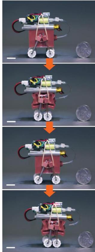
**Figure S7.** The soft robotic walker made untethered by carrying its own power supply, pump, valve, and circuit board. Scale bars are 1cm.
