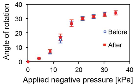
**Figure S9** Comparison of the angle of rotation vs. applied negative pressure curve of three single-unit buckling actuator samples fabricated in Elastosil before and after 1000000 cycles of actuation at 2Hz.
