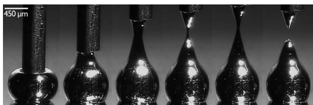
Figure 1. A series of photographs of the formation of a conical tip of EGaIn. From left to right: A micromanipulator 1) brings a drop of EGaIn suspended from the needle of a syringe into contact with the bare, reflective surface of an Ag film, and 2) raises the syringe until the EGaIn separates into a conical tip (which remains attached to the needle of the syringe) and a drop on the Ag surface. The pictures are sequential and show the formation of a single tip; the time spanned by this sequence is less than 5 s.
