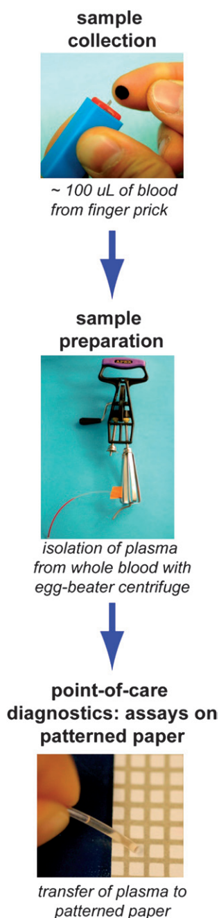
Fig. 1 Point-of-care diagnostics result in rapid, in-field diagnosis. Health workers can extract a small volume of blood from a finger prick and can load the blood into EDTA-coated, PE tubing. To prepare the sample for the diagnostic, plasma is isolated from whole blood using the hand-powered centrifuge.
