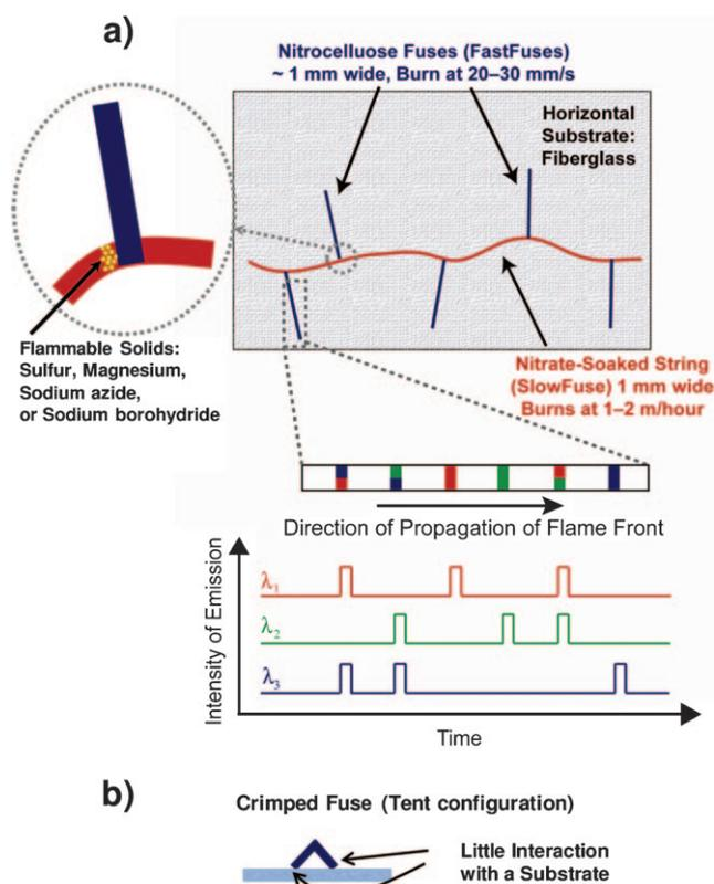
**Figure 1.** a) Diagram of a slow-burning, nitrate-soaked cotton string (SlowFuse), with appended fast-burning nitrocellulose fuses (Fast-Fuses) that transmit information as optical pulses of light characteristic of thermally emissive alkali metals. b) Diagram of a crimped fuse (tent configuration) with little interaction with a substrate.
