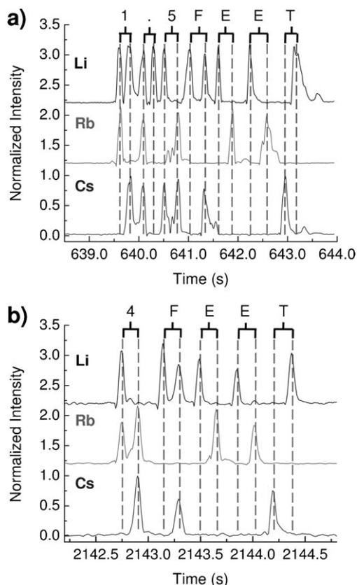
**Figure 3.** Transmitted light detected from a two-speed infuse when a) a FastFuse ignited after 1.5 feet of the SlowFuse had burned (10.6 min), and b) a FastFuse ignited after 4 feet of the SlowFuse had burned (35.7 min). In the encoding scheme used here, two consecutive optical pulses represent one alphanumeric character. The fuse burned on a glass wool and was ignited once at  $t = 0$  s.
