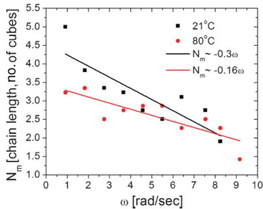
FIG. 4. (Color online) Peak position,  $N_m$ , vs angular velocity of the jar,  $\omega$ : squares and circles represent data from experiments conducted at room temperature and 80°C, respectively. The lines represent a best fit through the data with the gradient stated in the legend. This figure provides evidence for the predicted linear relationship between  $N_m$  and  $\omega$  and the dependence on the interaction energy.
