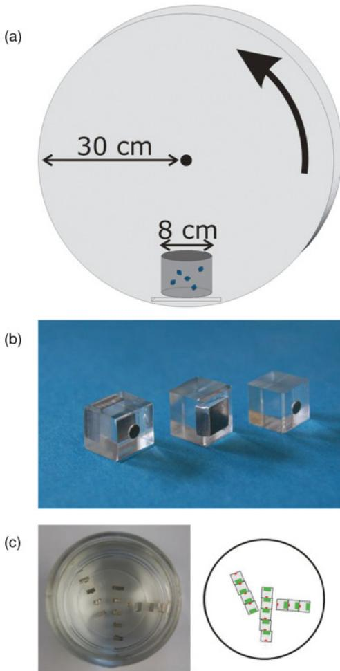
FIG. 1. (Color online) (a) Schematic sketch of the experiment.  $N$  cubes are placed in a closed container, which is then attached to a rotating disk that generates a turbulent flow. (b) Polydimethylsiloxane blocks with small embedded disk-shaped magnets and prism-shaped NiCu pieces. (c) Agitation in a turbulent flow causes the blocks to form chains; green (dark gray), NiCu pieces; red (light gray), magnets.
