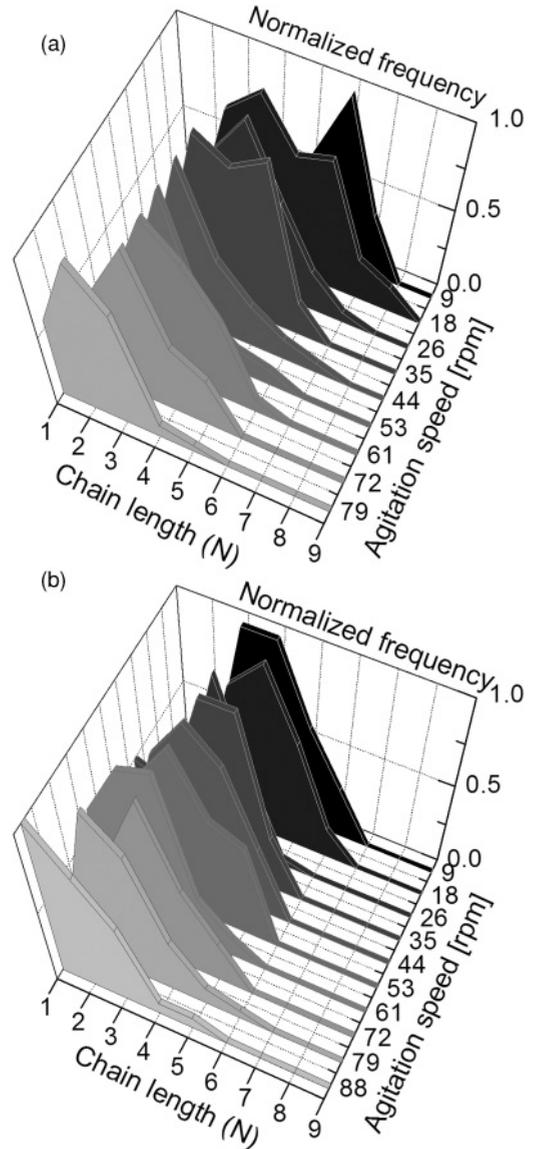
FIG. 2. Histogram of the distribution of chain lengths measured in the experiment, for a range of different rotation rates, and both (a) room temperature and (b)  $T = 80^\circ\text{C}$ . Changing the temperature shifts the strength of the magnetic interaction. The peak of the distribution shifts as a function of both temperature and rotation rate.
