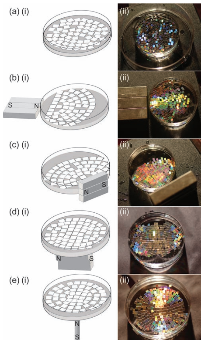
Figure 5. Packing structures of the tiles differed according to the pattern of magnetic field applied. a) The tiles in the absence of magnetic fields. The length and width of each tile were both 2 mm. b–e) The assembly of tiles in response to different patterns of magnetic fields.
