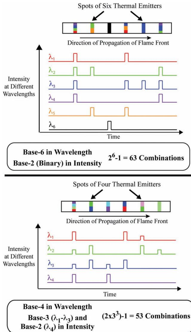
**Figure 1.** Schematic diagram of infuses that can encode and transmit alphanumeric information with individual optical pulses. Top: A schematic description of a binary system in intensity that uses six different thermally emissive salts. Bottom: A schematic description that is binary and ternary system in intensity and that uses four different thermally emissive salts.
