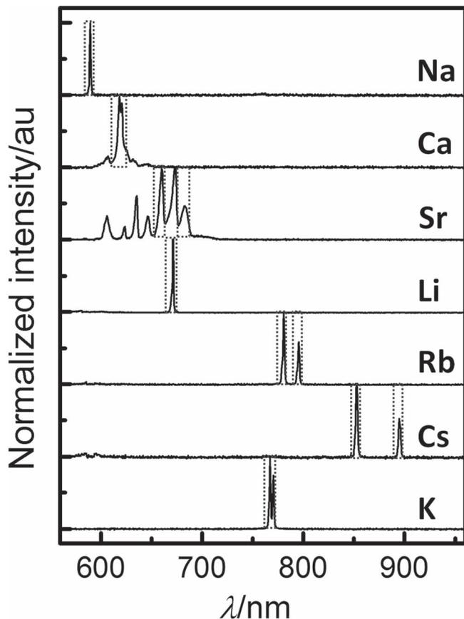
**Figure 2.** Normalized thermal emission spectra (between 550 and 950 nm) of sodium, calcium, strontium, lithium, rubidium, and potassium perchlorate deposited on a burning infofuse. The boxes with gray dashed borders show the areas of the emission spectrum that we integrated to determine the intensity of emission from each metal salt. We avoided overlaps between Sr, Ca, and Li by excluding combinations of Ca and Sr, and Li and Sr, as in Figure 3.
