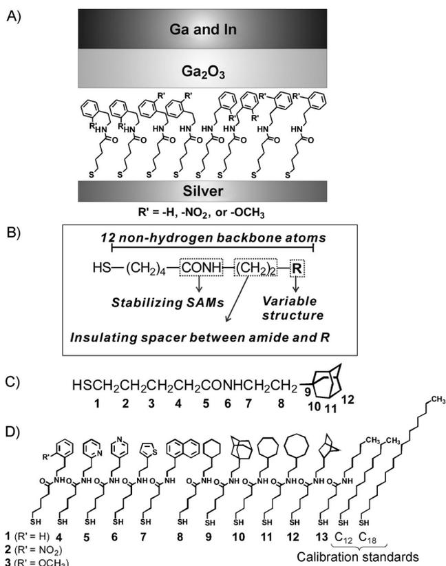
**Figure 1.** A) Schematic representation of a tunneling junction consisting of a template-stripped Ag bottom electrode supporting a SAM, and contacted by a  $\text{Ga}_2\text{O}_3/\text{EGaIn}$  top electrode. B) A schematic representation of one junction. C) The numbering system based on non-hydrogen atoms in the backbone of the molecules tested. D) Molecules used to form SAMs for this study.
