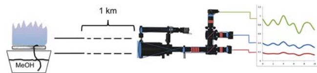
Figure 1. Atomic emission beacon composed of a cotton wick doped with one or more metal salts. Upon combustion of methanol, the metal ions become atomized and release characteristic emission that can be detected 1 km away using collection optics, bandpass filters, and photodiodes.
