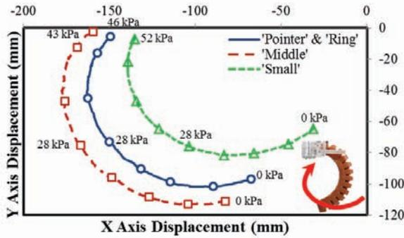
Fig. 8. Experimental tip displacement of all manufactured actuators. The actuators are horizontally aligned with the  $x$  axis and their free end starts bending in a clockwise fashion from point  $(0, 0)$ .
