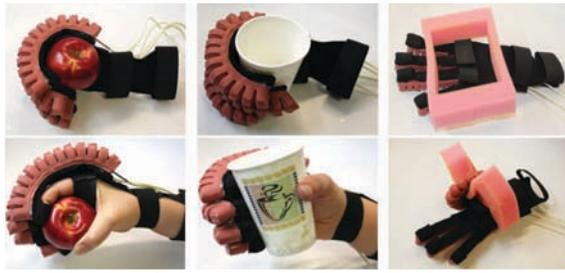
Fig. 11. Using the soft glove to grasp various objects.
