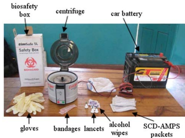
Fig. 5. Equipment for the SCD-AMPS rapid test. All the equipment necessary to run the rapid test in a rural clinic fits inside a backpack and were evaluated at rural health centers in Zambia.
