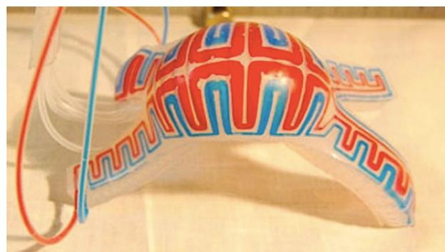
**Figure 6.** Cephalopods such as squid, octopuses, and cuttlefish use their ability to change colour to hide from predators. This soft robot uses simple microfluidic channels to camouflage its ‘skin’, hiding from detection in both the visible and infrared [23].
