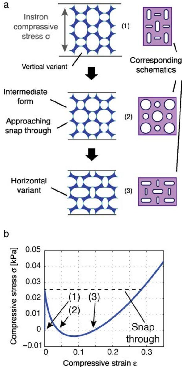
**Fig. 5.** Simulation of the switching behavior. (a) The ferroelastic phase in horizontal variant was realized by applying an external pressure (state (1)). A vertical compressive stress  $\sigma$  was then added. After an intermediate state (state (2)), the vertical variant switched to the horizontal variant (state (3)). (b) Simulated relation of the compressive stress  $\sigma$  and the compressive strain  $\epsilon$  of a unit cell during domain switching.
