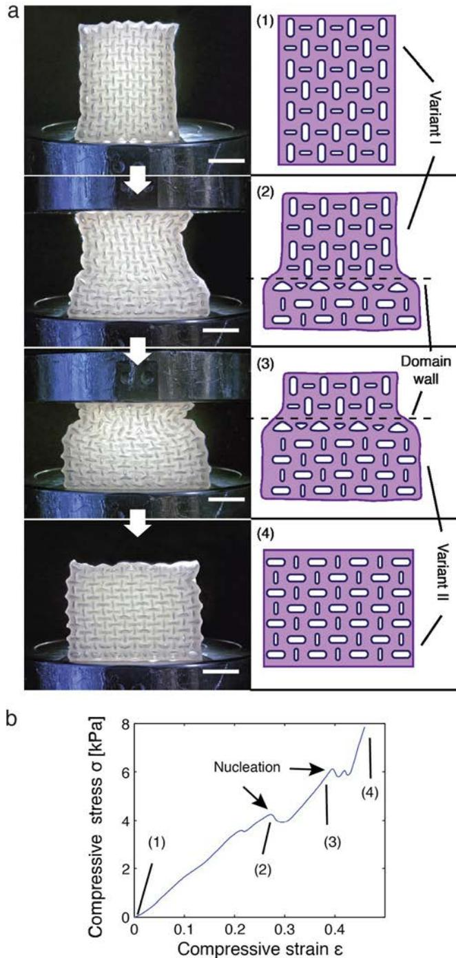
**Fig. 4.** Switching of the metamaterial (under atmospheric pressure) from the vertical variant to the horizontal variant in the ferroelastic phase on vertical compression. (a) By applying a compressive load in the long axis, the rectangular sample switches between its two variants. The spontaneous strain persists even after the removal of the load. (b) The bulk stress–strain curve of the rectangular sample during switching as recorded by Instron. The scale bars are 2 cm long.
