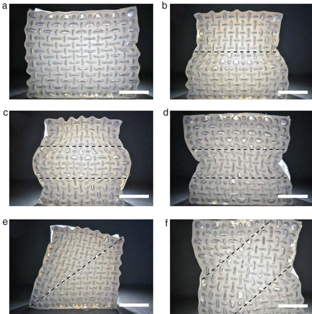
**Fig. 6.** Ferroelastic domain patterns. (a) A single-domain structure. (b) A two-domain structure with a horizontal domain boundary. (c, d) A three-domain structure with two horizontal boundaries. (e) A two-domain structure with a 45-degree domain boundary. (f) A three-domain structure with two 45-degree domain boundaries. Domain boundaries are marked with a dotted line. Scale bars are 2 cm long.
