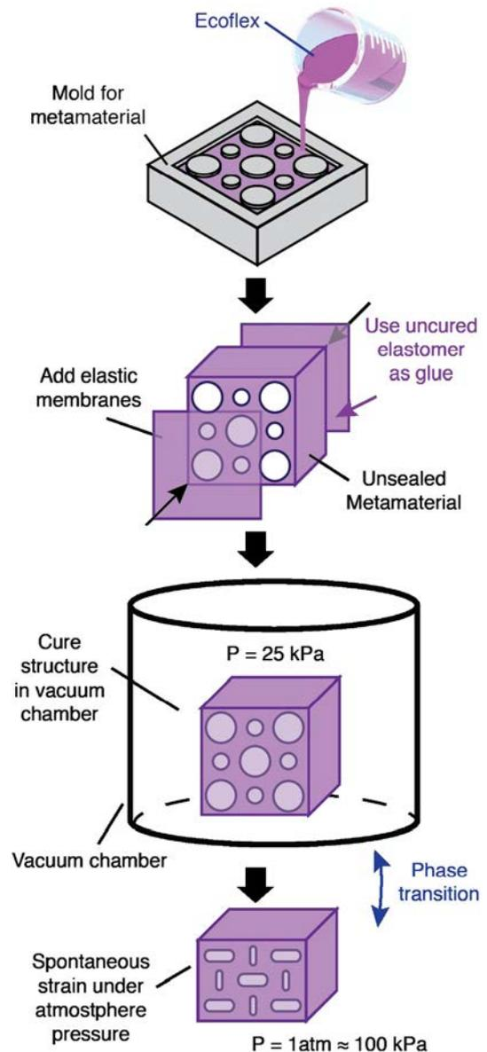
**Fig. 2.** Fabrication of the ferroelastic metamaterial. First, we cast Ecoflex into a 3D printed mold to generate the desired structure. The elastomeric slab containing the array of holes was then removed from the mold. Two thin sheets of Ecoflex were used to cover the holes, and the structure glued and cured at reduced pressure (25 kPa). When the completed structure was removed from the vacuum chamber, it underwent a phase transition from the parent phase to the ferroelastic phase.
