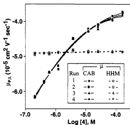
**Figure 5.** Change in the electrophoretic mobilities of CAB and HHM on increasing the concentration of 4. Four replicates were run for this experiment and are labeled as 1–4 in the legend.
