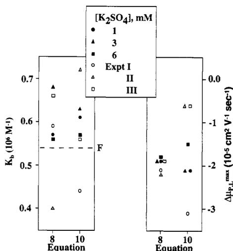
**Figure 2.** Values of binding constants  $K_b$  and  $\Delta\mu_{P,L}^{\max}$  of 1 and CAB with addition of potassium sulfate to induce changes in electroosmotic flow and the value obtained by a fluorescence assay (F).
