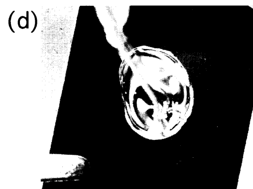
Figure 2. Potential-dependent wetting of an aqueous solution of electrolyte (10 mM \text{CH}_3(\text{CH}_2)_2\text{SH} , 0.1 M \text{NaClO}_4 , 5 mM \text{K}_2\text{HPO}_4 , 5 mM \text{KH}_2\text{PO}_4 , pH 7) on a gold film patterned with self-assembled monolayers of \text{CH}_3(\text{CH}_2)_2\text{S} and \text{CH}_3(\text{CH}_2)_{15}\text{S} : (a) schematic illustration of the patterned surface; photograph (top view) of liquid at (b) E = 0 \text{ V} (Ag wire), (c) E = -1.4 \text{ V} , and (d) E = 0 \text{ V} . The photographs in the sequence (b–d) were taken approximately \sim 30 \text{ s} apart. The reference electrode was a 0.5 mm diameter Ag wire and the counter electrode was a 0.25 mm Pt wire.
