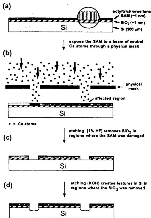
FIG. 1. Schematic diagram of the experimental procedure (not to scale). (a) A SiO<sub>2</sub> substrate was first coated with a SAM of octylsiloxane. (b) The substrate was then exposed to a beam of neutral cesium atoms through a physical mask. (c) In a wet-chemical-etching step, the pattern of damage caused by the cesium was transferred into the SiO<sub>2</sub> layer. (d) Finally, the SiO<sub>2</sub> pattern was used as a mask for etching into the underlying Si substrate.
