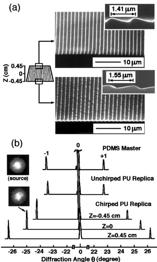
*Figure 11* (a,b) Cross-sectional SEM images of selective regions of a planar, chirped, and blazed PU replica grating that was fabricated by molding against a PDMS mold while it was compressed asymmetrically (22). The PDMS mold was prepared by casting against a commercial blazed diffraction grating. (c) Diffraction patterns from the PDMS mold, its PU replica, and the chirped PU grating. A He-Ne laser ( $\lambda = 632.8$  nm) was used.
