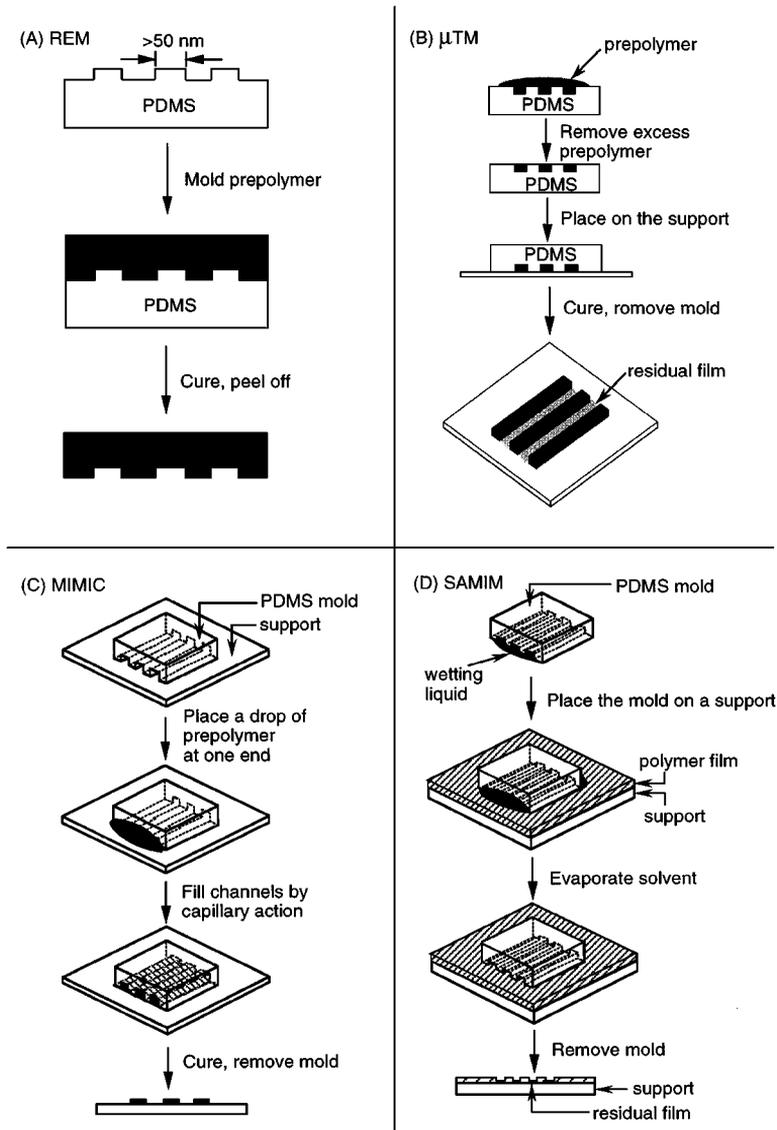
Figure 5 Schematic illustration of procedures for (a) replica molding (REM), (b) microtransfer molding ( $\mu$ TM), (c) micromolding in capillaries (MIMIC), and (d) solvent-assisted micromolding (SAMIM).
