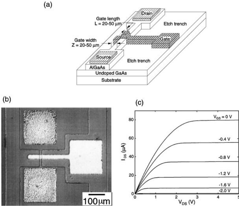
Figure 12 (a) Schematic diagram of a GaAs/AlGaAs FET. (b) Optical micrograph of a GaAs/AlGaAs FET ( $L = 26 \mu\text{m}$  and  $Z = 16 \mu\text{m}$ ) fabricated using MIMIC (182). (c) The performance of a representative GaAs/AlGaAs FET fabricated using this procedure.
