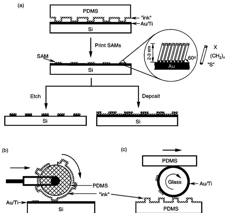
Figure 2 Schematic procedures for  $\mu$ CP of hexadecanethiol (HDT) on the surface of gold: (a) printing on a planar surface with a planar stamp (21), (b) printing on a planar surface over large areas with a rolling stamp (128), and (c) printing on a nonplanar surface with a planar stamp (174).
