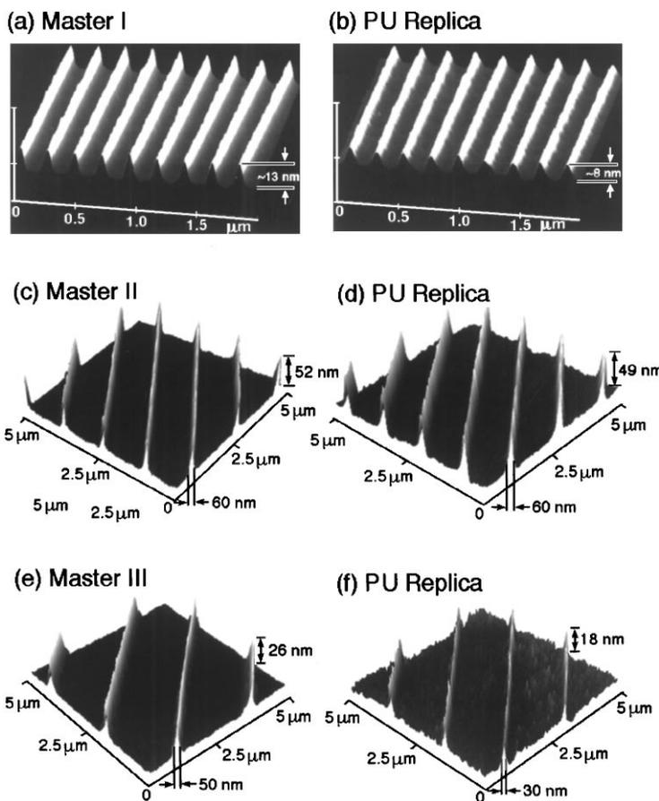
*Figure 6* (a,b) Atomic force microscopy (AFM) images of Cr structures on a master, and a PU replica prepared from a PDMS mold cast from this master (153). (c,d) AFM images of Au structures on another master, and a PU replica produced from a PDMS mold cast from this master. (e,f) AFM images of Au structures on a third master, and a PU replica fabricated from a PDMS mold (cast from this master) while this mold was mechanically deformed by bending in a manner that generated narrower lines.
