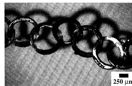
Fig. 4. Optical micrograph of a free-jointed nickel chain formed by the procedure shown in Fig. 3. The final thickness of nickel was \sim 50 \mu\text{m} .
