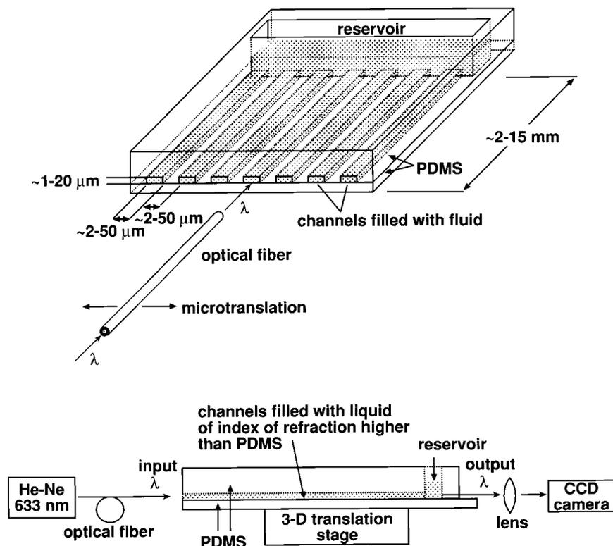
Fig. 3. Schematic diagram of the optical coupling set-up using an optical fiber to couple light into liquid-core waveguides. High index fluid trapped in micron-sized channels by capillarity guide light by total internal reflection. The output of the channels is imaged with a CCD camera.
