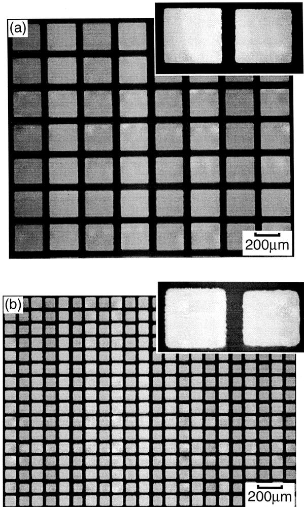
Fig. 2. SEM micrographs of arrays of Schottky diodes with contact areas of (a) 200  $\mu\text{m} \times 200 \mu\text{m}$  and (b) 80  $\mu\text{m} \times 80 \mu\text{m}$ . Both arrays were fabricated using  $\mu$ TM. The insets in (a) and (b) are magnified views of single Schottky diodes corresponding to the two contact sizes.
