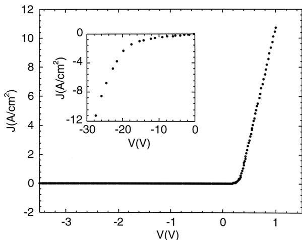
Fig. 3. Current density vs. applied voltage of a representative Schottky diode with contact area  $200\ \mu\text{m} \times 200\ \mu\text{m}$  fabricated using  $\mu\text{TM}$ . The inset is the reverse breakdown characteristics of the Schottky diode.
