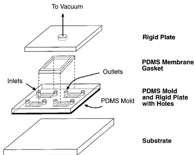
Fig. 1. Schematic illustration of the setup used in vacuum-assisted MIMIC with multi-point inlet design. Prepolymer was applied at the outer holes and the vacuum was applied at a single point near the center. The multi-point inlet design combined with vacuum-assisted MIMIC allowed rapid filling of capillaries over a large area.
