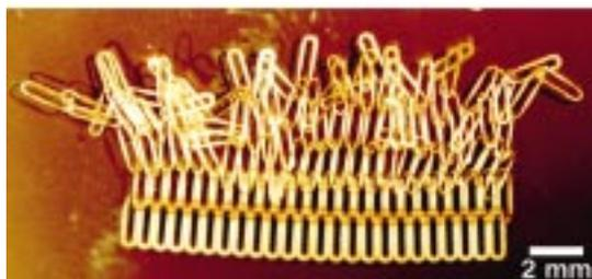
Figure 2. Top: A freely interlocked chain mail (5 × 24 ovals) fabricated by using one glass slide and five cylinders; bottom: a blow-up image of the chain mail.
