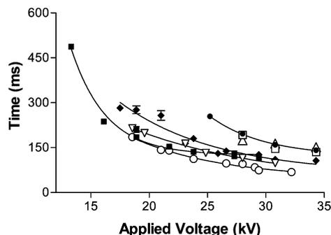
**Fig. 5** Problem solving time measured as a function of the applied voltage for: a straight line 2 mm long (■) at 27 torr, a straight line 13.5 mm long (▽) at 24 torr, a simple maze (○) at 27 torr, a complex maze (◆) at 159 torr, route from Imperial College to Buckingham Palace (●), route from Imperial College to Victoria Station (□) and route from Imperial College to Big Ben (△) all at 486 torr.
