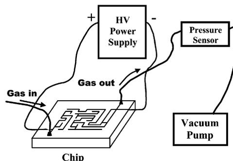
**Fig. 2** Schematic layout of the experimental setup used to produce the glow discharge in the chips. The tungsten wires, used as electrodes (not shown), are introduced through the channels adjacent to the starting and ending points. The helium gas is introduced through the inlet capillary connected to the chip and is evacuated through the outlet capillary connected to the pressure sensor and vacuum pump.
