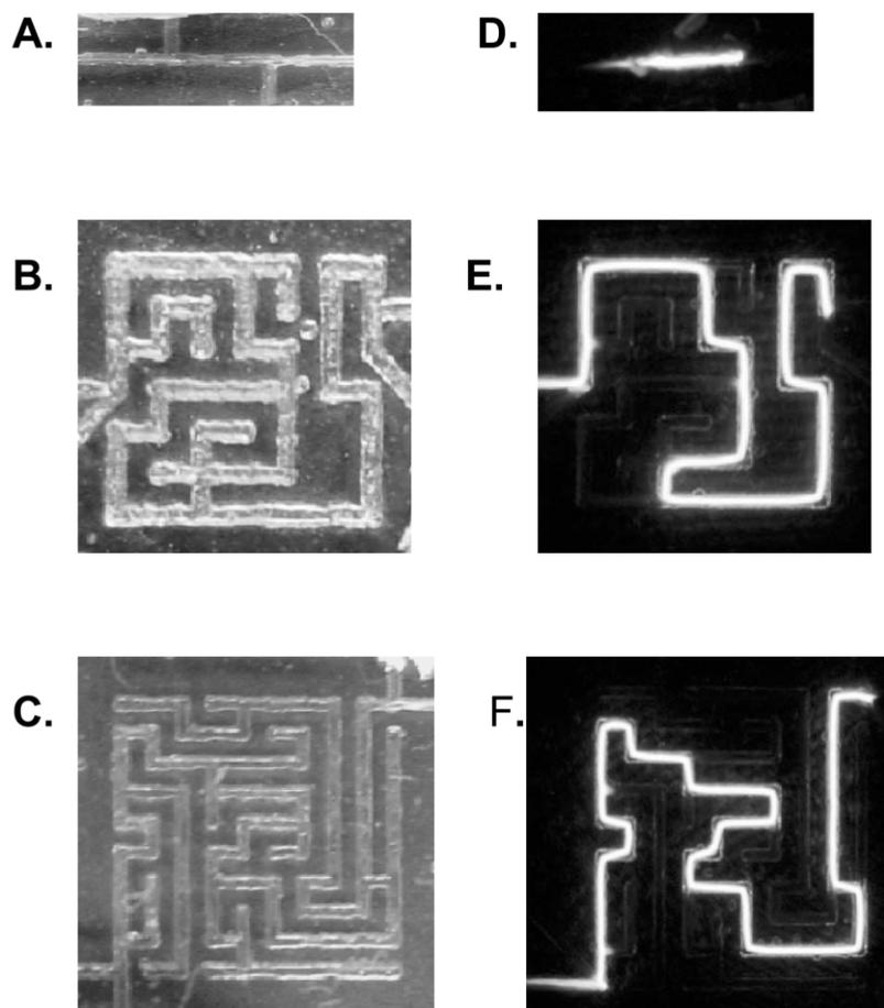
**Fig. 3** Images of (A) a straight channel, (B) a maze and (C) a maze of higher complexity. (D) A glow discharge in (A) when 1.12 kV is applied at 11 torr. (E) Image of glow discharge showing the route for the shortest path in the maze (12 torr and 4.02 kV). (F) Image of the glow discharge showing the route from one end to the other of a more complex maze (5.77 kV and 161 torr).
