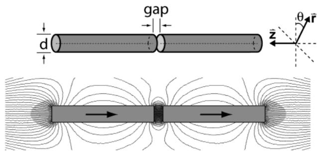
**Figure 1.** (top) Schematic of a metallic rod of diameter  $d$  comprising two ferromagnetic regions (gray) separated by a gap. To the right is a coordinate system representing the axial ( $z$ ) and radial ( $r$ ) directions. (bottom) Magnetic simulation of the field surrounding a cross section of the rod. The contours represent the field lines; the shading represents magnetic flux density,  $\mathbf{B}$ .
