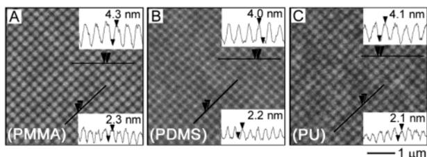
**Figure 2.** AFM images of (A) PMMA test structures generated by writing a grid of crossed lines with an electron beam ( $\sim 200$  electrons/nm<sup>2</sup>, 30 kV), (B) the corresponding mold in *h*-PDMS, and (C) a PU replica. The parallel lines, spaced by 250 nm, are  $\sim 2$  nm deep except where the lines intersect with a depth of  $\sim 4$  nm.
