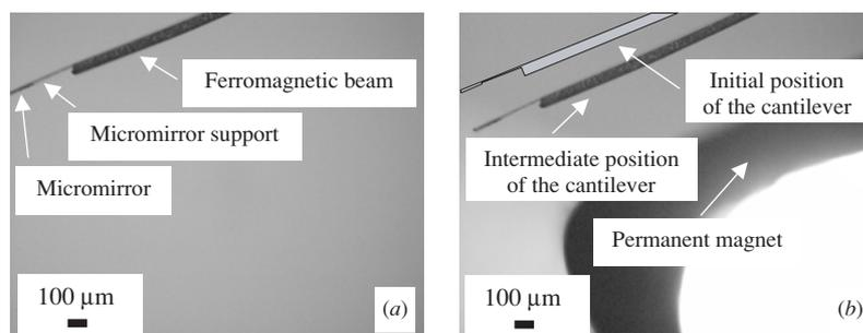
**Figure 7.** (Side view) Deflection of the tip of the cantilever as the permanent magnet approached. The micromirror was positioned at the tip of the cantilever on the supporting platform. The other end of the cantilever was anchored (not shown in the figures). (a) Initial position of the cantilever. (b) Intermediate position of the cantilever and of the permanent magnet.
