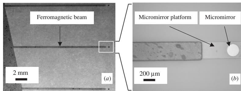
**Figure 5.** (Top view) Optical microscope images of the magnetically actuated micromirrors after release. (a) A set of three cantilevers, 10 mm, 11 mm and 12 mm long. The micromirrors are at the end of each cantilever. (b) Close-up image of the end of a cantilever, showing the circular micromirror and the supporting platform.
