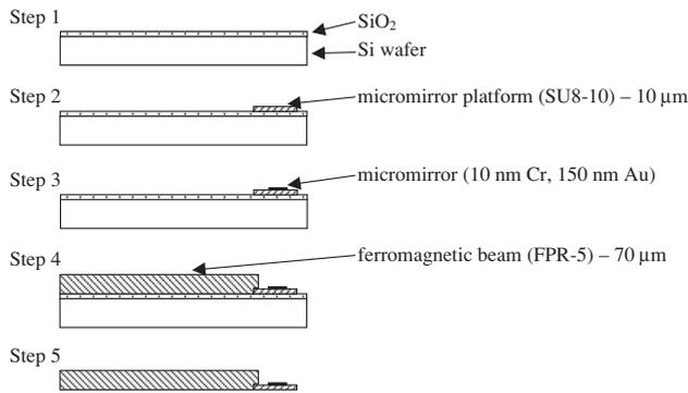
**Figure 4.** Cross-section of the fabrication process for the magnetically-actuated micromirror. Main steps include: (1) thermal growth of silicon dioxide; (2) patterning the micromirror platform; (3) forming the micromirror; (4) fabricating the beam from FPR and (5) releasing the cantilever.
