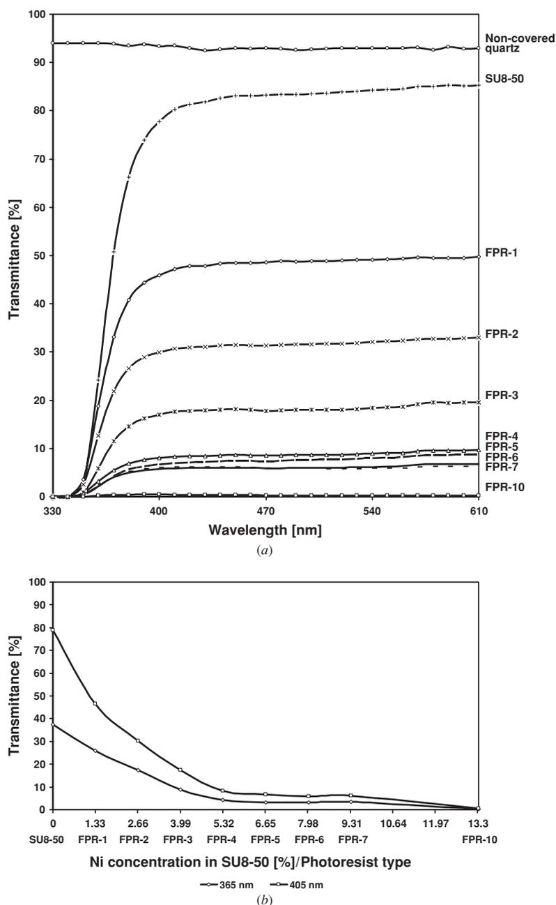
**Figure 3.** (a) Measured transmittance of 70  $\mu\text{m}$  thick FPR- $n$  ( $n = 0, 1, \dots, 7$ , and 10) on quartz disks. Five points on each disk were measured; the deviation between these measurements was less than 2% for each wavelength (not shown in the figure). (b) Measured transmittance of processed FPR- $n$  at wavelengths 365 nm (I-line) and 405 nm (H-line) as a function of the nickel concentration (data extracted from figure 4(a)).
