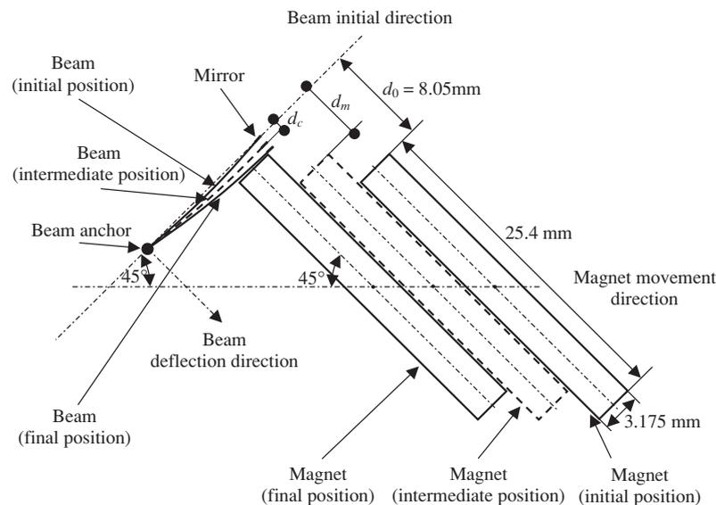
**Figure 6.** Sketch of the experimental set-up for the determination of the deflection of the cantilever versus displacement of the permanent magnet. In the final position of the magnet, the magnet is in physical contact with the cantilever.
