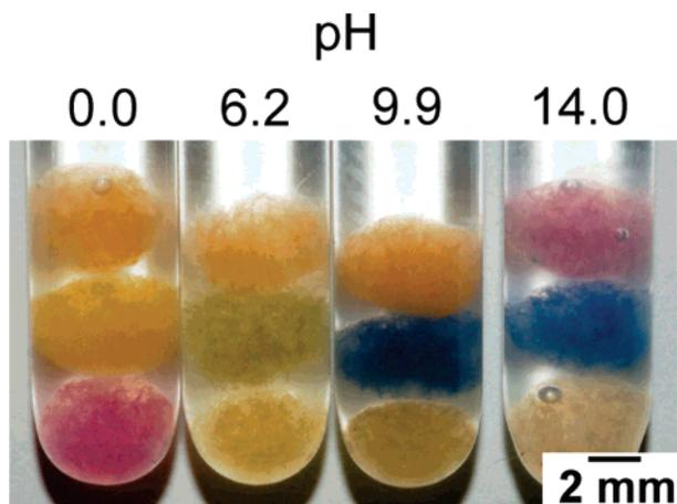
**Figure 4.** Optical image of the same set of three types of hydrogel spheres with embedded fibers of pH paper containing different covalently bound indicators in solutions titrated to four different values of pH: 0, 6.2, 9.9, and 14 (from left to right). Each tube contains three spheres (one of each set).
