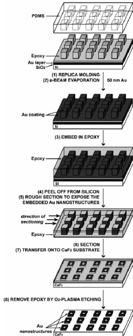
**Figure 1.** Schematic illustration of the procedure used to fabricate arrays of approximately square loop-shaped nanostructures on a solid substrate (e.g.,  $\text{CaF}_2$ ). Square structures are fabricated by isotropic coating of square posts with gold by electron-beam evaporation, followed by nanoskiving. Fabrication of L- and U-shaped nanostructures is accomplished starting with the same square posts and depositing Au by shadow evaporation.
