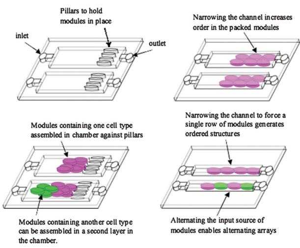
Fig. 1 Schematic suggesting the assembly of modules in a microfluidic chip.
