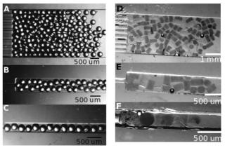
**Fig. 3** Templated packing of hard and soft objects in microchannels. Glass beads (260  $\mu$ m wide) in microchannels (A) 2 mm, (B) 500  $\mu$ m, and (C) 250  $\mu$ m wide. The beads were most ordered when confined to the narrowest channels. Agarose cylinders (150  $\mu$ m diameter, 300  $\mu$ m long) in microchannels (D) 2 mm, (E) 500  $\mu$ m, and (F) 150  $\mu$ m wide also showed more order in narrow channels than in wide ones.
