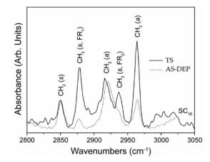
Figure 6. Plots of the C-H stretching region of the RAIR spectra for the SAMs of SC16 on TS silver and on AS-DEP silver. The spectra were smoothed by five-point adjacent averaging. The symmetric and asymmetric methylene stretching peaks are at higher energies for SAMs on AS-DEP silver than for SAMs on TS silver, an indication that the SAMs on AS-DEP silver are less ordered than those on TS silver.
