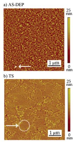
Figure 5. Contact-mode AFM images of the topography of the (a) AS-DEP silver film and (b) TS silver film. The root-mean-square roughnesses of a 25  $\mu$ m<sup>2</sup> area of the silver films are 5.1 ± 0.4 nm for AS-DEP and 1.2  $\pm$  0.1 nm for TS. The white circles indicate the approximate size of the largest grains in each film and have diameters of (a) AS-DEP, 80 nm, and (b) TS, 1 µm.
