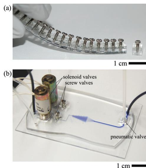
**Fig. 4** (a) A photograph of a strip of prefabricated screw valves. A single valve has been separated from the strip using a razor blade. (b) A photograph of a microfluidic gradient generator containing two embedded solenoid valves, two embedded screw valves and one embedded pneumatic valve. The design of this device is shown in Fig. 8.
