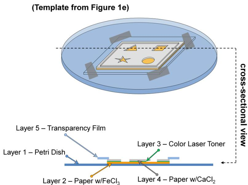
**Figure S2.** A schematic diagram showing the steps for the fabrication of gels with step-gradients in the concentration of cross-linking ions. A sheet of chromatography paper with a printed layer of toner (a) was cut into shaped pieces (b). We turned these pieces over and wet them with solutions of salts at different concentrations (c) and juxtaposed the pieces with ~2 mm of overlap. A 2% solution of sodium alginate applied to the template (d) gelled into a single continuous film (e).
