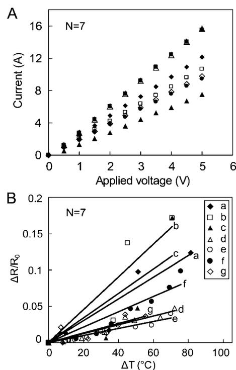
**Fig. 3** Electrical properties of carbon resistors. (A) Linear current–voltage curves for carbon resistors ( $N = 7$ ), showing the ohmic  $I$ – $V$  characteristics of a good conductor. The slope of the current–voltage curve represents the resistance of the carbon resistor. (B) Calibration plot of the relative change in resistance as a function of the change in temperature.
