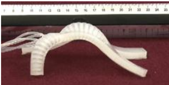
Video S3. Real time video of soft robot crawling using high modulus (Ecoflex 00-50 ©) pneu- nets.
