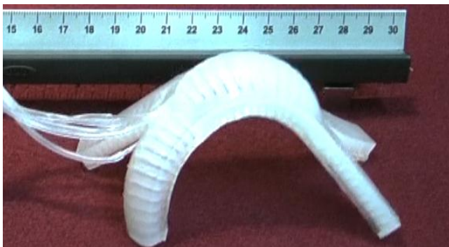
Video S3. Real time video of soft robot crawling using high modulus (Ecoflex 00-50 ©) pneu- nets.
