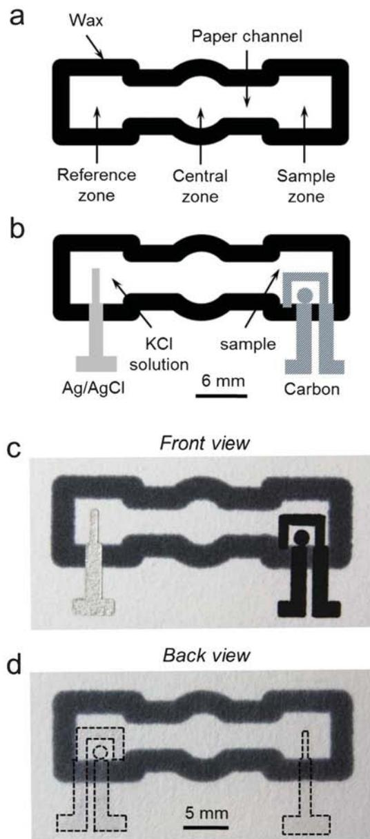
**Fig. 1** Schematic illustrations (a and b) and photographs (c and d) of a referenced Electrochemical Paper-based Analytical Device (rEPAD). The paper was patterned by wax printing to define the sample zone, central contact zone, reference zone, and microfluidic channels. The sample and reference zones include stencil-printed carbon and Ag/AgCl electrodes, respectively. The dashed lines in (d) indicate the approximate boundaries of the carbon and Ag/AgCl ink printed on the back.
