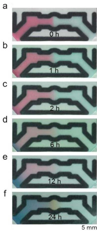
**Fig. 2** Photographs of a sealed paper-based microfluidic device taken after the addition of a pink aqueous solution of  $\text{CoCl}_2$  and a blue solution of  $\text{CuSO}_4$  to the left and right zones, respectively. The two solutions mixed in the central zone but did not diffuse into the right or left paper zones. The color of the  $\text{CoCl}_2$  solution became paler after 1 h and changed to blue after 12 h as water in the device gradually evaporated.
