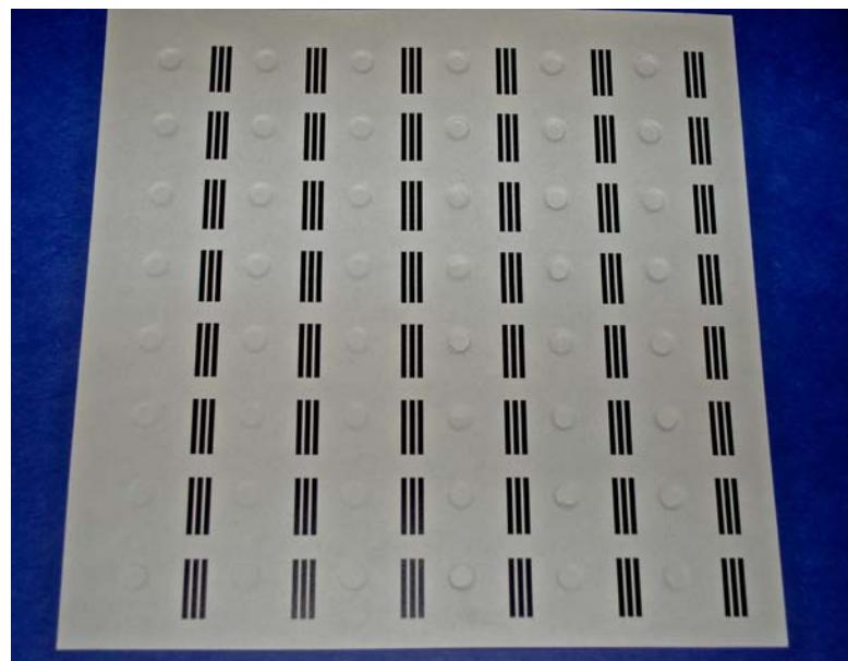
**Figure S1:** A “48 well plate” comprising 48 individual electrochemical cells. The diameter of each well is 7 mm.
