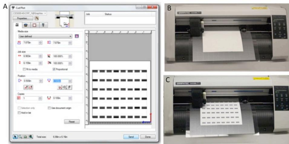
**Figure S3:** Printing of electrodes using a pen filled with conductive graphite ink and a desktop cutter-plotter (Craft ROBO Cutting plotter). (A) The electrode design is loaded into ROBO Master, the software that controls the output of the plotter; B) the plotter with the paper loaded; c) the plotter prints the electrode onto the surface of the paper. The entire process takes less than 8 min for 48 electrodes.
