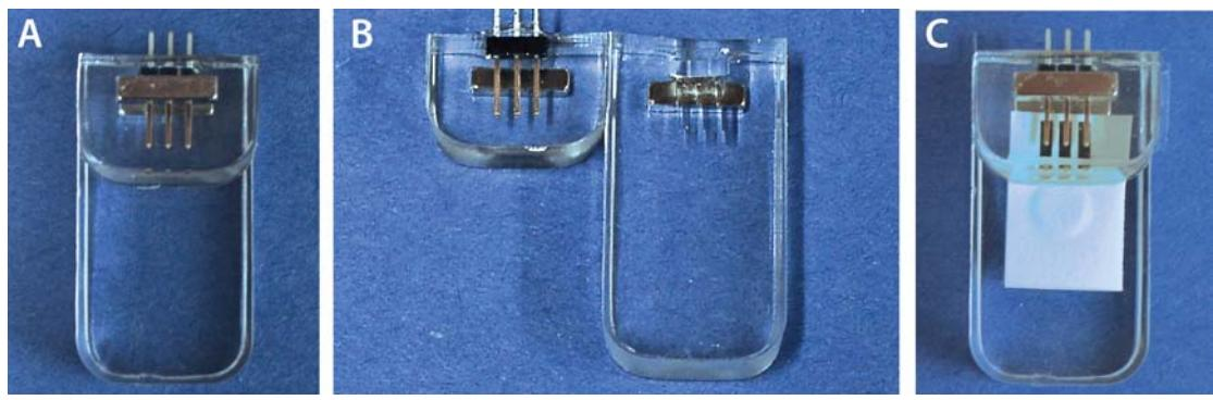
**Figure S4:** PDMS holder (A) consisting of two PDMS parts with embedded magnets (B). The holder can be used to connect the three electrodes (RE, WE and CE) of the electrochemical cell with the cable leads of a potentiostat (C).
