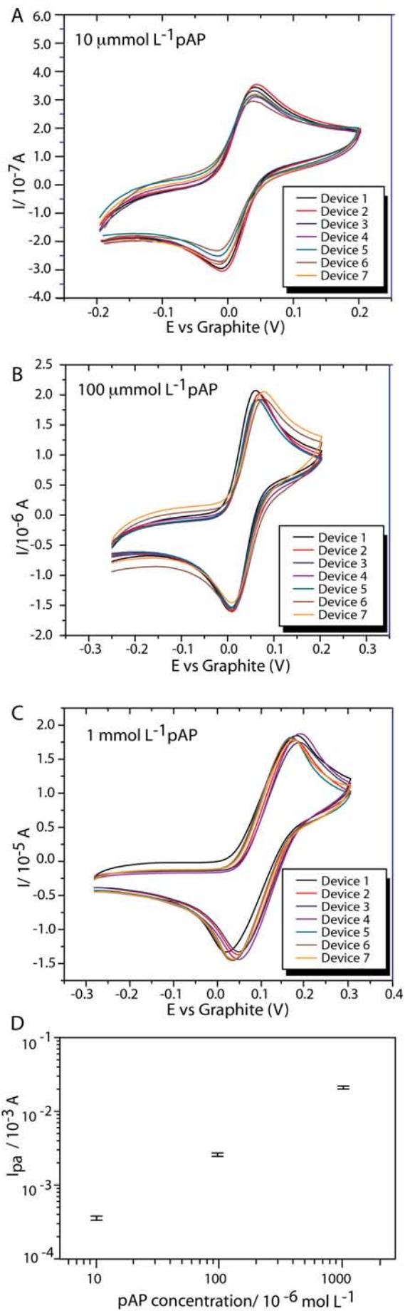
**Figure S6.** A-C) Cyclic voltammograms of pAP for a range of concentrations for seven devices prepared in different batches. D) Plot of relation between pAP concentration and measured anodic peak current (CV); the scales for both concentration and peak current are logarithmic. Each datum represents the average of seven independent measurements, and the error bars represent the standard deviation from the average.
