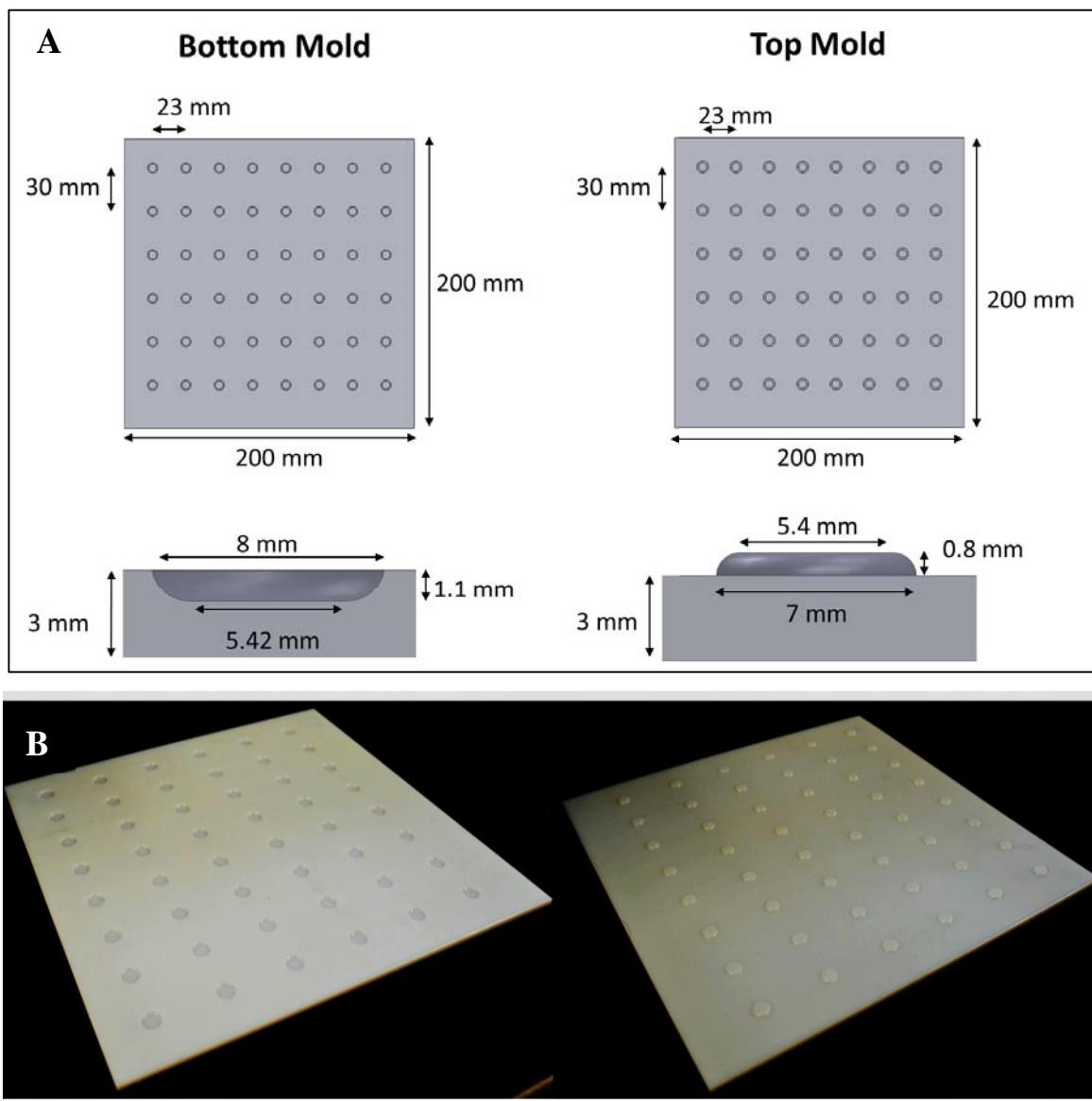
**Figure S2:** (A) Characteristic dimensions of the features in the molds used for embossing. (B) Image depicting the 200×200 mm molds used to emboss the “48 well plate”. Left: negative mold. The diameter of each feature is 8 mm; the depth of each feature is 1.1 mm. Right: positive mold. The diameter of each feature is 7 mm; the height of each feature is 0.8 mm.
