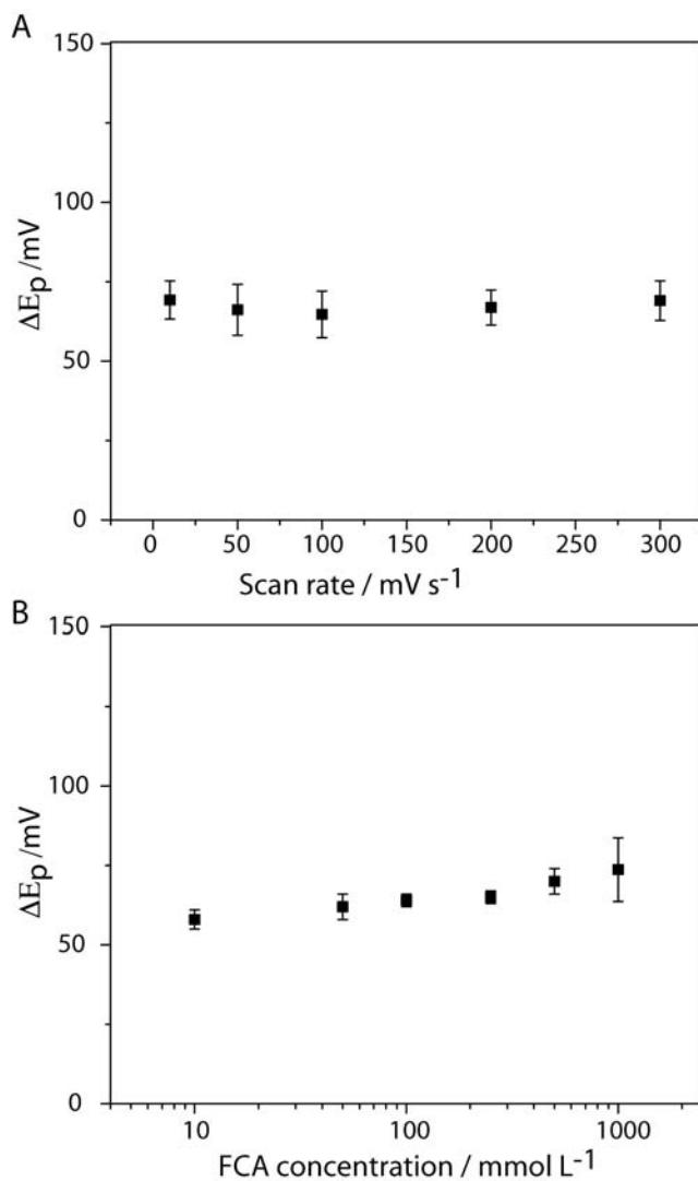
**Figure S7.** Variation of the peak current potential separation  $\Delta E_p = E_{pa} - E_{pc}$  with: (A) scan rate, for a  $100 \mu\text{mol L}^{-1}$  solution of FCA in PBS, pH 7.6; (B) concentration of FCA in PBS, pH 7.6, at a scan rate of  $100 \text{ mV s}^{-1}$ . In (B), the x-axis is logarithmic.
