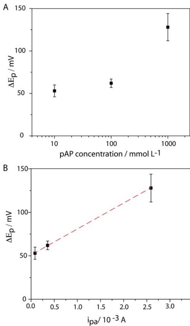
**Figure S8.** Variation of the peak current potential separation  $\Delta E_p$  with: (A) concentration, and (B) peak current measured for three concentrations of pAP [1 mmol L<sup>-1</sup>, 100  $\mu$ mol L<sup>-1</sup>, 10  $\mu$ mol L<sup>-1</sup>] in PBS, pH 7.6, at a scan rate of 100 mVs<sup>-1</sup>. In (A), the x-axis is logarithmic.
