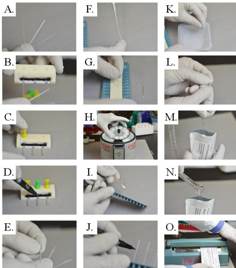
A silicone sleeve slides over the tube to open or close the hole. Using a pipette, we load a pre-mixed solution of an SCD-AMPS solution into the tube from one end and then seal that end with white, vinyl-based polymer sealant (Critoseal, Leica).
