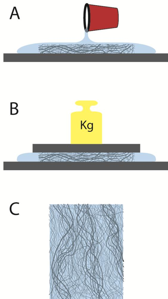
**Figure S2.** Fabrication of a CEC Sheet. (A) A sheet of metal wool was placed on a metal plate and soaked in uncured elastomer. (B) The soaked metal wool sheet was cured in an oven while being pressed by a top metal plate and additional weights. (C) The cured product was trimmed with scissors to generate the final CEC sheet.
