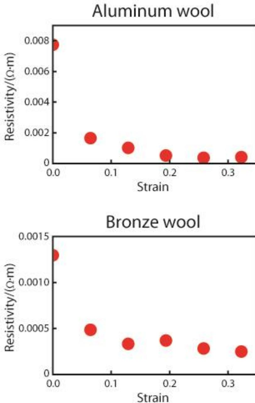
**Figure S3.** Resistivity Measurements. Plot of resistivity vs. strain for two representative CEC sheets made from aluminum wool (Top) and bronze wool (Bottom). The sheets were elongated in the direction perpendicular to the majority fiber axis as current was transmitted in the same direction as the elongation. Strain data is provided based on measurements of engineering strain.
