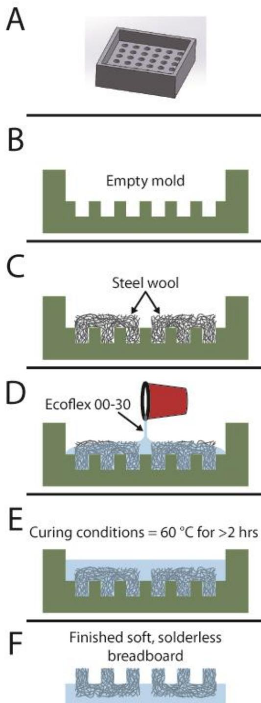
**Figure S10.** Fabrication of the Soft, Solderless Breadboard. (A) Perspective view of the mold. (B) Cross section of the mold before part fabrication. (C) Placement of steel wool to create conductive paths and connectors for electrical components. (D) Addition of uncured elastomer. (E) Curing of the elastomer. (F) Finished soft, solderless breadboard.
