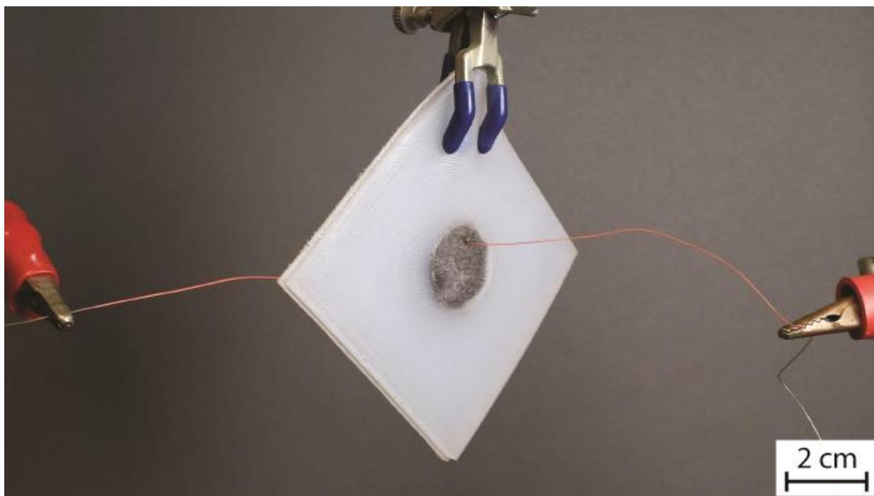
**Figure S4.** Creating a Conductive Path. Photograph of an elastomeric sheet with a disk shaped steel wool conductive CEC path at its center. For this demonstration, resistive nickel-chromium wires were inserted into the two opposing faces of the CEC to provide a visual indication of the flow of electrical current. The CEC is passing a current of 2.5 A across the elastomeric sheet as evidenced by the blackbody radiation being emitted from the wires used to supply and drain the current.
