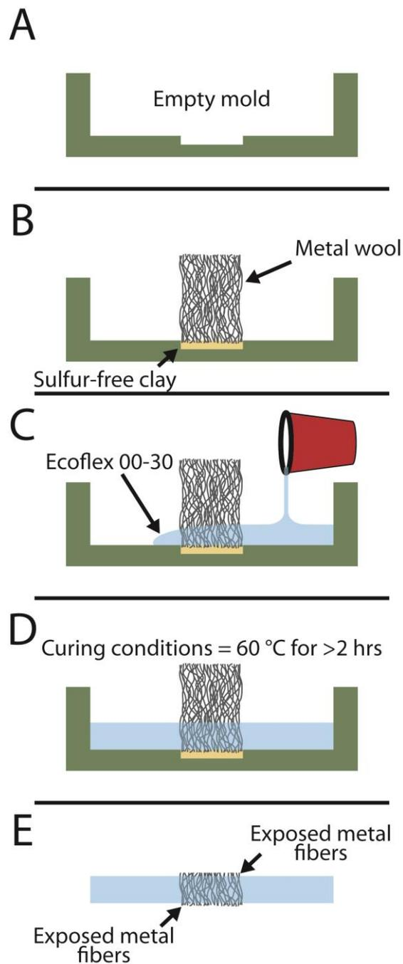
**Figure S8.** Fabrication of an Elastomeric Sheet with a CEC Path as used for Figures S4, S5, S6, and S7. (A) Illustration of the empty mold. (B) A steel wool slab was inserted into a clay filled recession at the center of the mold. The clay was used both to position the slab and to prevent coating of the end of the slab with elastomer. (C) Filling of the mold with uncured elastomer. (D) Curing of the elastomer. (E) Final elastomeric sheet with steel wool CEC path.
