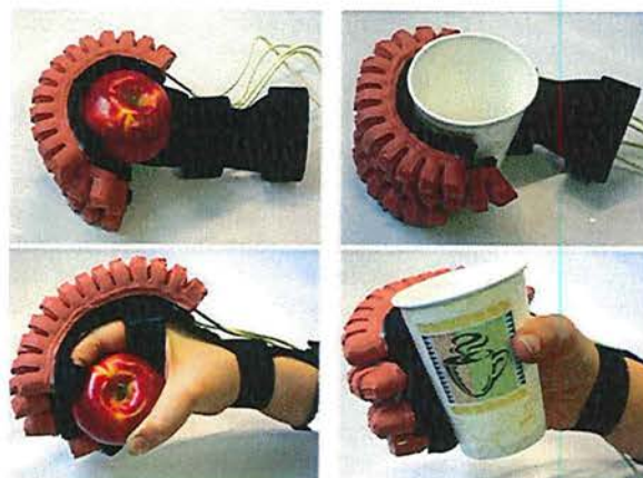
Figure 10. A grip-assist device, comprising a glove with pneumatically actuated elastomeric “fingers” that augment the grip of human fingers, or replace it. Reproduced from Ref. [68] with permission. Copyright 2013, IEEE Proceedings.
