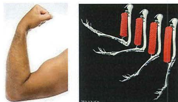
Figure 5. Left: Human arm showing the biceps muscle. Right: a PneuNet structure that combines negative (sub-atmospheric) pressure and reversibly buckling elastomeric beams to mimic the function of this muscle. [43] Reproduced from Ref. [43] with permission. Copyright 2016, John Wiley & Sons.
