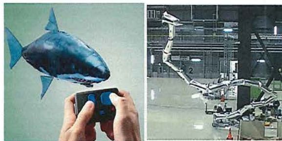
Figure 9. Light-weight structures (essentially, structured helium-filled balloons). Left: A commercial children's toy (an “air swimmer”). Right: A long, steerable arm (a Giacometti Arm with a 20-m balloon body). Suzumori Endo Lab, Tokyo Institute of Technology. [66]
