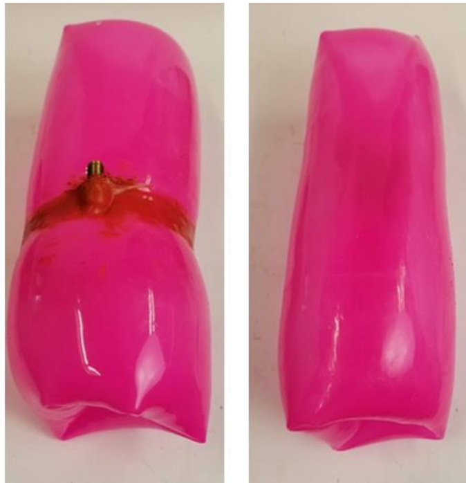
Figure S2. Photograph of an air-filled toroidal hydrostat containing a Schrader valve. Shown with the valve facing outwards (left) and inwards (right).
