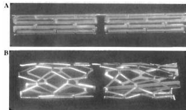
Fig. 4. Unexpanded (A) and expanded (B) structures with the dimensions of Palmaz-Schatz coronary stents generated by electroplating silver onto silver structures formed on glass capillaries with  $\mu\text{CP}$ . The glass was removed with concentrated HF after electrodeposition.
