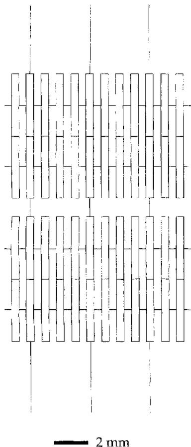
Fig. 2. Negative illustration of the amplitude photomask used to form the stamps for producing structures with the dimensions of a Palmaz-Schatz coronary stent. The lines are 20  $\mu\text{m}$  wide and correspond to raised regions of the stamp formed by this procedure. Lines extending from the top and the bottom parts of this pattern were used for electrical connection during the electrodeposition step, and were later removed with a razor blade.
