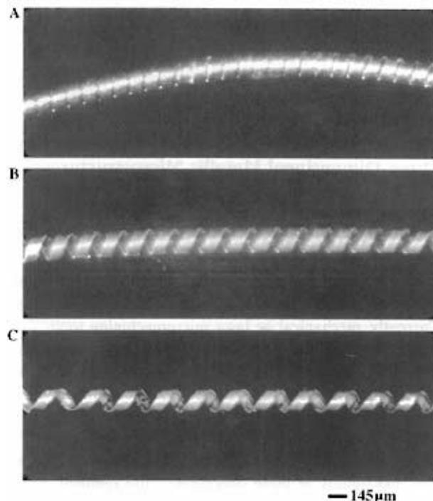
Fig. 3. Undeformed (A), elastically deformed (B), and inelastically deformed (C) micro-coil springs generated by electroplating silver onto silver micro-coils formed on glass capillaries with  $\mu\text{CP}$ . The glass was removed with concentrated HF after electrodeposition.
