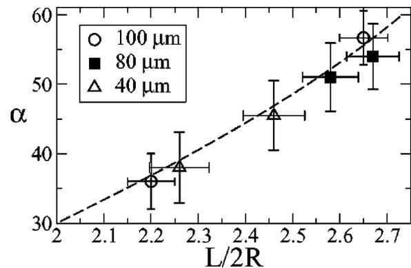
FIG. 3. Variation in angle  $\alpha$  versus normalized channel width  $L/2R$  for lattices containing three particles in the repeating unit. The dashed line shows the variation in  $\alpha$  estimated from Fig. 1(b).
