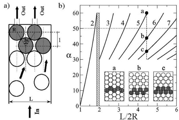
FIG. 1. (a) Flow-driven organization of spherical particles in a microchannel. The shaded beads constitute the repeating unit. The interlayer spacing  $l$  is shown on the right. (b) Diagram of possible regular phases obtained for particles with radius  $R$  for different values of  $L/2R$ . Each solid line corresponds to a given number of particles  $n$  in a repeating unit. In the dashed area no regular structures can be formed. Inset: Possible lattices obtained for  $L/2R = 4.46$ .
