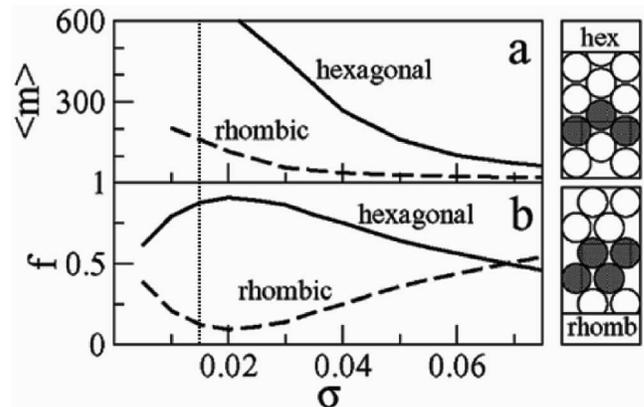
FIG. 5. Results of numerical experiments for channel width  $L/2R = 2.7$  for close-to-hexagonal (solid line) and rhombic (dashed line) structures: The average number of particles in a regular domain (a) and the fraction of beads in a lattice (b) are plotted versus the standard deviation  $\sigma$  in particle diameter. The vertical dotted line corresponds to the standard deviation of the beads used in the experiments.
